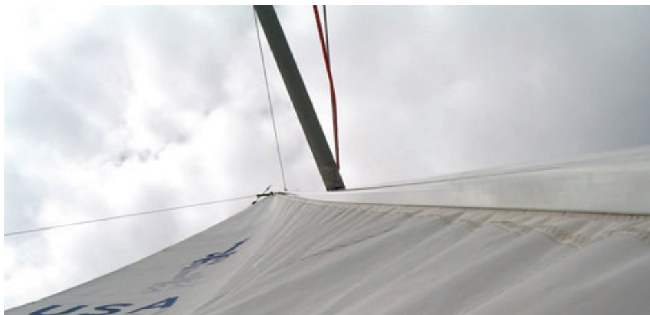
1"-3/4" of sag to leeward indicated proper lower shroud tension
