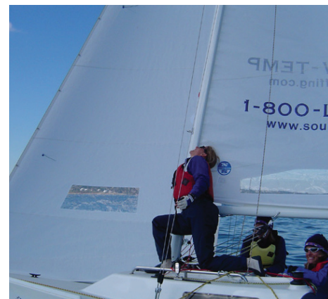
Sight the sag in the mast by sighting up the back of the mast when sailing upwind.
