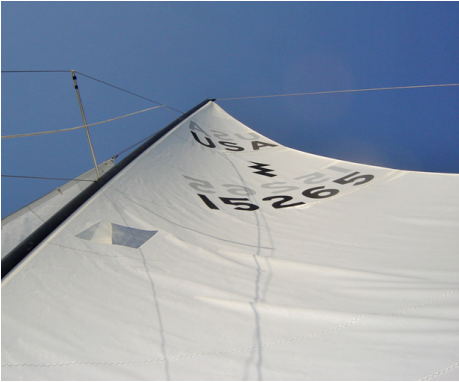
Too much backstay tension will create over bend wrinkles above the spreader window. Ease the backstay until they just disappear.
