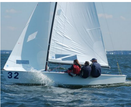
Ideally, over bend wrinkles will fall just below the spreader window and halfway back on the boom when proper prebend and mast bend is achieved.
