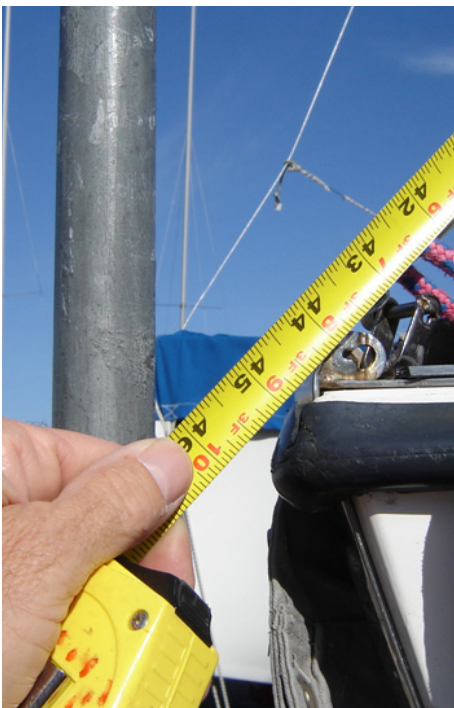
Measure from the top of the mark on your forestay to the joint of the bow and your deck to set your forestay length.
