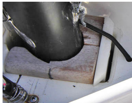
Usually a 1/2" block will be in place in front of the mast with the Fisher tuning with the New Allen and New Nickels boats.
