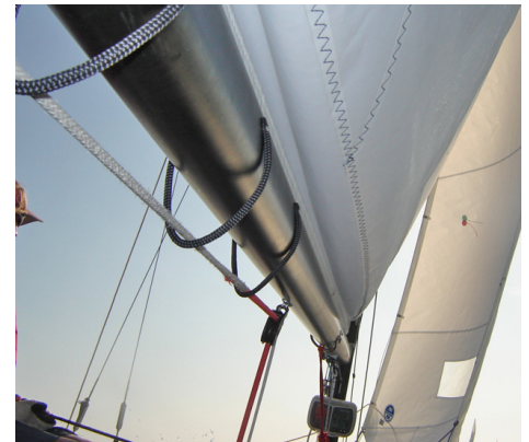
Use the shelf foot seam as a guide for outhaul tension.
