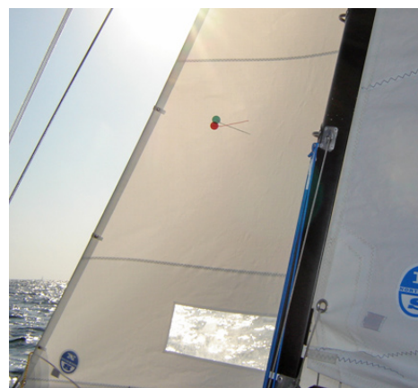
In breeze, set your jib cloth tension so the luff is smooth.
