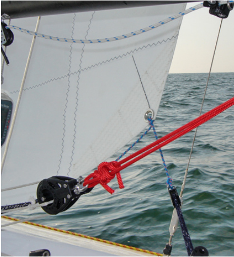
Set your jib lead in most conditions so the sheet is an extension of the trim line drawn on the clew.
